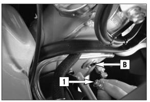
Fill 0.6 liters of engine oil into the can and remove the plug [1] next to the steering head. Introduce the plastic hose into the vent hole [B], (see page 30) and fill 0.6 liters of engine oil into the frame's front tube. Remove plastic hose, start engine, and let it idle (approx. 20 seconds) until oil escapes at the hole [B]. As soon as oil starts to escape, turn off the engine, and mount the plug together with the gasket and tighten to 25Nm.
