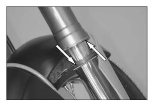
Clean dust-protection bellows, outer tubes, and fork tubes thoroughly, and oil them thoroughly with Universal oil spray (Motorex Joker 440) or engine oil. Then, push dust-protection bellows into the outer tubes by hand.
