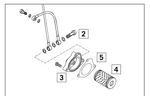
Place the new oil filter [4] on the connection in the oil filter cover and mount together with a new seal [5]. Tighten the 3 screws in the filter cover to 5 Nm (4 ft.lb). Tighten the hollow screw with seals and tighten to 15 Nm (11 ft.lb). Finally, start the engine and check the oil system for leakage.
