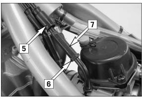
If a correction is necessary, start by removing the tank. Slide back the protection cover [5]. To set the backlash, loosen the counter nut [6] and turn the adjusting screw [7] accordingly. Then, fasten the counter nut and slide the protection cover back on.
