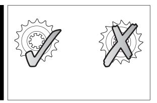
Also check sprockets and chain guides for wear, and replace if necessary.
