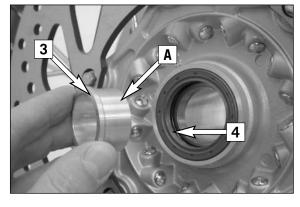
Before remounting the front wheel, clean and grease the shaft seal rings [4] and the bearing surface [A] of the distance bushings and mount the distance bushings (wide distance bushing in the left shaft seal ring). Slightly push back the brake pads with a screwdriver. Position the front wheel against the brake disks according to the direction of travel (see arrow [B]).
