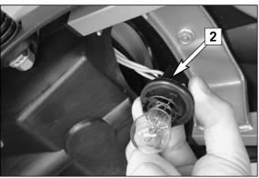
Turn the lamp socket [2] approximately 30° counterclockwise and pull it out of the tail light housing.
