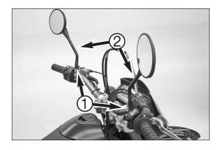
Mount both mirror supports ① and the mirrors ② (left hand thread), tighten the nuts.
