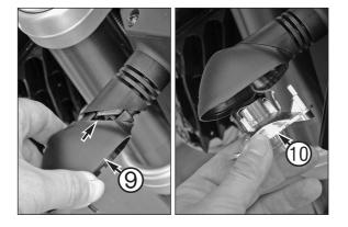
Mount right *and* left spoiler (the longer screw with washer use for position **3**).
