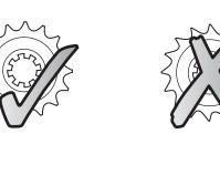
Also check sprockets and chain guides for wear, and replace if necessary.
