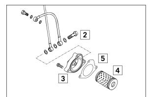
Place the new oil filter **[4]** on the connection in the oil filter cover and mount together with a new seal **[5]**. Tighten the 3 screws in the filter cover to 5 Nm (4 ft.lb). Tighten the hollow screw with seals and tighten to 15 Nm (11 ft.lb). Finally, start the engine and check the oil system for leakage.
