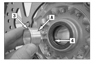
Before remounting the front wheel, clean and grease the shaft seal rings **[4]** and the bearing surface **[A]** of the distance bushings and mount the distance bushings (wide distance bushing in the left shaft seal ring). Slightly push back the brake pads with a screwdriver. Position the front wheel against the brake disks according to the direction of travel (see arrow **[B]**).
