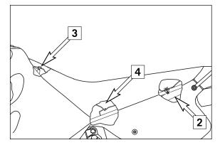
To install the seat, hook the seat into the oval-head screw, set the rear portion down on the frame, and slide it forward. If necessary, press down on the front area of the seat so that the seat catches on the retaining bracket **[4]**. Insert and tighten the collar screw.
