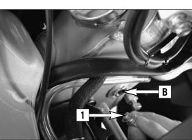
Fill 0.6 liters of engine oil into the can and remove the plug **[1]** next to the steering head. Introduce the plastic hose into the vent hole **[B]**, (see page 30) and fill 0.6 liters of engine oil into the frame's front tube. Remove plastic hose, start engine, and let it idle (approx. 20 seconds) until oil escapes at the hole **[B]**. As soon as oil starts to escape, turn off the engine, and mount the plug together with the gasket and tighten to 25Nm.
