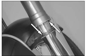
Clean dust-protection bellows, outer tubes, and fork tubes thoroughly, and oil them thoroughly with Universal oil spray (Motorex Joker 440) or engine oil. Then, push dust-protection bellows into the outer tubes by hand.
