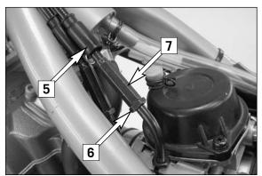
If a correction is necessary, start by removing the tank. Slide back the protection cover [5]. To set the backlash, loosen the counter nut [6] and turn the adjusting screw [7] accordingly. Then, fasten the counter nut and slide the protection cover back on.
