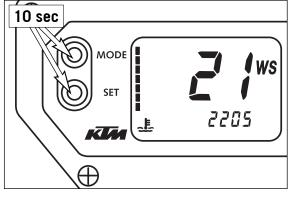
The preset wheel diameter  $(21, 19 \text{ or } 17^{"})$  and the respective wheel circumference (2205, 2040 or 1882 mm) are displayed briefly when the ignition is switched on.
