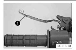
The clutch lever **①** is fitted on the left side of the handlebar. The clutch is hydraulically operated and self-adjusting.
