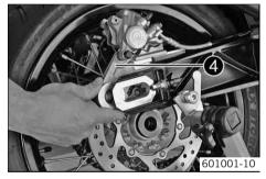
Pull the rear wheel and brake caliper support 4 together to the rear until you can swing the brake caliper support to the side.
