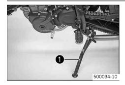
The side stand lacktriangle is coupled with the safety electric starter system - see the riding instructions.
