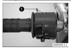
The headlight flasher switch **1** is fitted on the left side of the handlebar.
