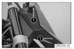
Remove the 4 screws **1** and carefully take off the headlight mask.
