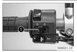
The turn signal switch • is fitted on the left side of the handlebar.
