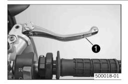
The hand brake lever **①** is fitted on the right side of the handlebar. The front brake is engaged using the hand brake lever.
