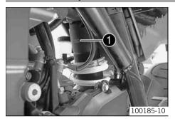
The shock absorber part number  $oldsymbol{0}$  is stamped on the top of the shock absorber above the adjusting ring on the engine side.
