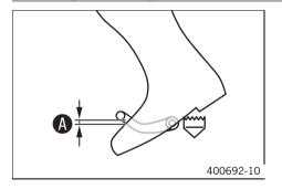
Sit on the vehicle in the riding position and determine the distance between the upper edge of your boot and shift lever .
