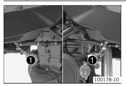
The fuel taps **1** are located on the left/right under the fuel tank.
