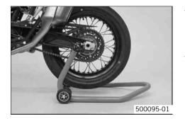
Insert the work stand adapter in the work stand and screw it into the link forks.
