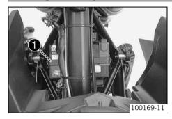
Push the battery from the right into the battery rack.
