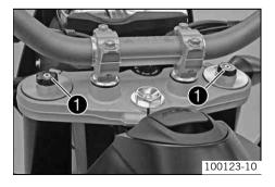
Turn adjusting screws • clockwise all the way.
