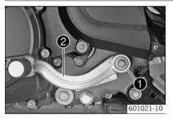
Remove screw 1 and remove shift lever 2.
