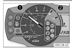
The tachometer • shows the engine speed in revolutions per minute.
