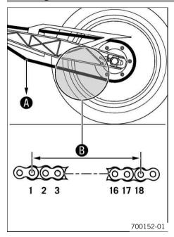
Shift into neutral, pull the lower chain section with the specified weight .
