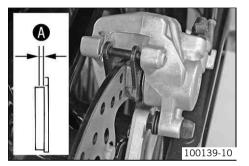
Check the brake linings for minimum thickness **(4)**.
