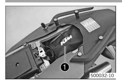
The tool set **1** is located in the storage compartment under the seat.
