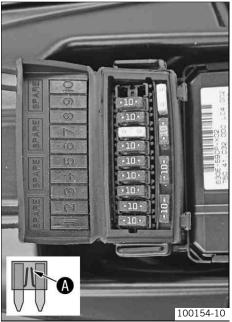
Remove the faulty fuse.
