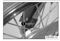
The fork part number **1** is stamped on the inner side of the fork stub.
