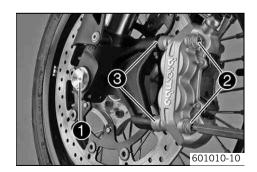
Clean and grease the thread of the wheel spindle and screw •.
