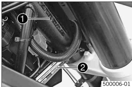
The chassis number ❶ is stamped on the right of the steering head.
