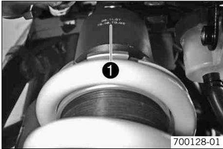
The shock absorber part number ❶ is stamped on the top of the shock absorber above the adjusting ring toward the rear.
