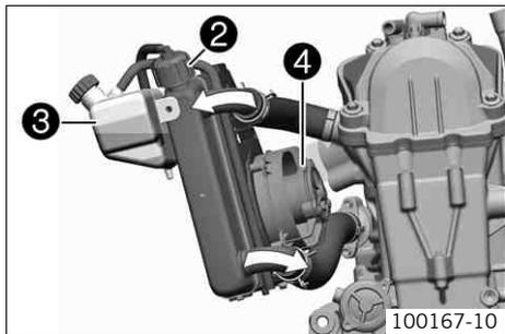
The coolant is cooled by the air stream and a radiator fan ❹, which is controlled by a thermostat.
