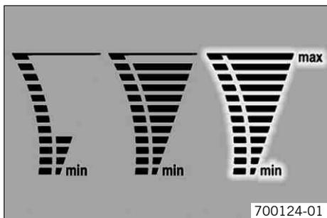
The temperature display consists of 12 bars. The more bars showing, the hotter the coolant. When the top bar lights up, all bars begin to flash and the temperature warning light starts to show.
