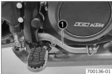
The footbrake pedal ❶ is located in front of the right footrest. The footbrake pedal operates the rear brake.
