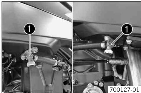
The fuel taps ❶ are located on the left/right under the fuel tank.
