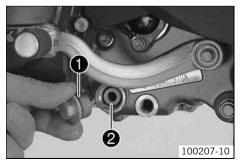
Remove plug **1** with oil screen **2** and the O-rings.
