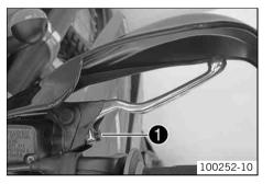
Adjust the free travel of the handbrake lever with the adjustment screw **①**.
