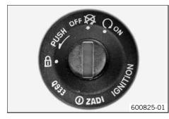
The ignition/steering lock **1** is in front of the upper triple clamp.
