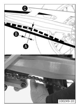
Adjusting the chain tension
