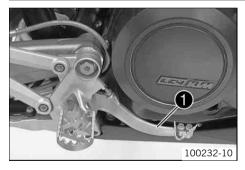
The footbrake pedal  $\bullet$  is located in front of the right footrest. The footbrake pedal operates the rear brake.
