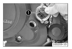
Remove the oil filler plug with O-ring ① from the clutch cover and fill up with engine oil.
