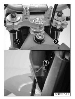
Position the headlight mask and fix it with rubber band 2.
