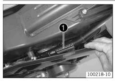
Type label **1** is located on the upper right frame tube below the seat.
