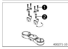
Remove the four screws ①. Remove the handlebar clamp. Remove the handlebar and lay it to one side.
