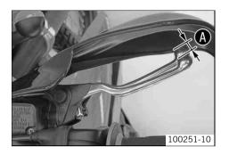
Push the hand brake to the handlebar and check free play **(4)**.
