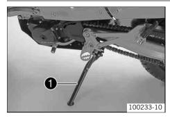
The side stand  ${\pmb 0}$  is coupled with the safety electric starter system - see the riding instructions.
