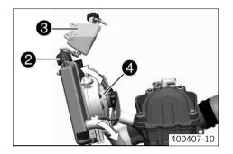
The coolant is cooled by the air stream and a radiator fan ④, which is controlled by a thermoswitch.
