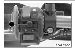
The flasher switch • is fitted on the left side of the handlebar.
