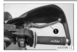
The hand break lever **①** is fitted on the right side of the handlebar. The hand brake lever operates the front brake.
