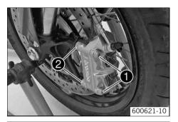
Position the brake calipers. Install the screws • with the spacers •.
