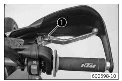
Adjust the basic setting of the handbrake lever to your hand size by turning adjusting wheel ①.
