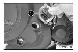
Remove filler plug with O-ring 1 from the clutch cover and add engine oil.
