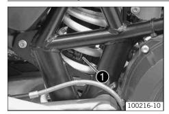
The shock absorber part number **1** is on the right of the shock absorber.
