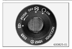
The ignition/steering lock • is located in front of the seat.
