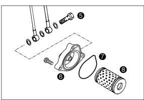
The O-ring need not be replaced unless it is damaged. Press the O-ring into the groove of the oil filter cover, mount a new oil filter on the oil filter cap and mount the unit. Insert the 3 screws and tighten them with 5 Nm (4 ft.lb). Mount the banjo bolt with the gaskets and tighten it with 15 Nm (11 ft lb)
