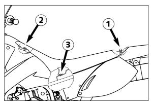
When installing the seat, be sure to insert the rear portion of the seat into the metal clasp  $\ensuremath{\mathfrak{G}}$ .
