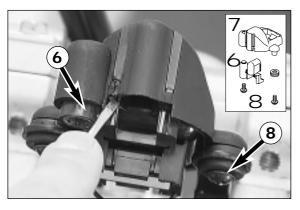
Use a screwdriver to lever the blue speedometer glass 6 downward and out of the speedometer housing 7. The two noses A must be disengaged from the speedometer housing. Remove screws 8, and take speedometer out of housing.
