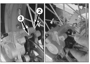
Slide left brake pad into the brake caliper and fix it with the pin. Slide in the right brake pad and knock the bolt in as far as it will go. Mount safety device 2.
