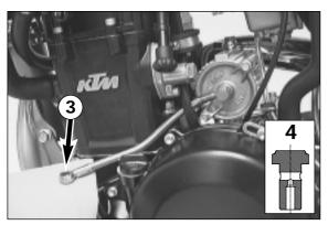
It is necessary to bleed the micro filter so that all friction areas can be quickly supplied with engine oil. To do this, fill with oil and remove the jet screw 4 from the oil line on the clutch cover. Start the engine and close off the oil filler hole on the clutch cover with a rag. Allow the engine to run at idle until oil runs out of the oil line 3. Turn the engine off. Install seal rings and the jet screw. Torque the jet screw to 10 Nm (7 ft.lb) and check for
