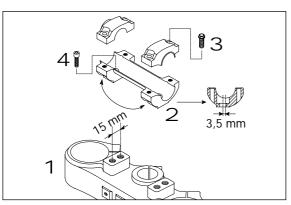
For this purpose, remove screws 3 of the handlebar clamps and screws 4 of the handlebar support. Position handlebar support, and tighten screws 4 to 40 Nm (30 ft.lbs). Mount handlebar and handlebar clamps, and tighten screws 3 to 20 Nm (15 ft.lbs). The gap between handlebar support and handlebar clamps is to be of equal size in the front and in the rear.
