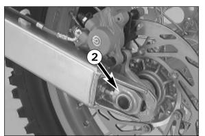
The rear wheel is remounted in reverse order. Before tightening the collar nut to 80 Nm (59 ft.lb), push the rear wheel forwards so that the chain tensioners lie on the tension screws.
