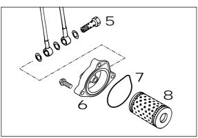
The O-ring 7 need not be replaced unless it is damaged. Press the O-ring into the groove of the oil filter cover, mount a new oil filter 8 on the oil filter cap and mount the unit. Insert the 3 screws and tighten them with 5 Nm (4 ft.lb). Mount the banjo bolt with the gaskets and tighten it with 15 Nm
