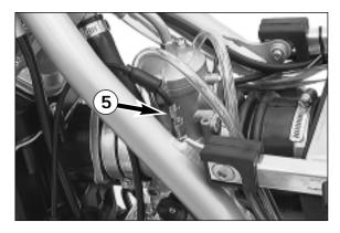
To adjust, remove the seat and the gastank, push the protective cover upwards, loosen the counter nut and turn the adjustment screw 5 accordingly. Turn the adjustment screw clockwise for more play or anticlockwise for less play.
