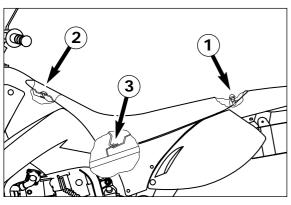
When installing the seat, be sure to insert the rear portion of the seat into the metal clasp  $\ensuremath{\mathfrak{Z}}$ .
