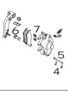
Mount the right brake pad and fix it with the bolt. Mount the left brake pad and insert the bolt until it stops. Mount the clips.
