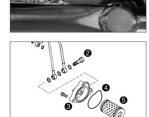
Check the O-ring **④** for damage. O-rings need not be replaced unless damaged. Press the O-ring into the groove of the filter cover. Fit new oil filter **⑤** with rubber gasket on the fitting in oil filter cover and mount cover with filter. Mount three screws and tighten with 5 Nm (4 ft.lb). Mount hollow screw with seal rings and tighten with 15 Nm (11 ft.lb). Start engine and check oil system for leakage.
