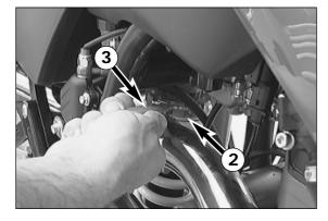
Loosen the allan head screw **1** at the adjustment ring **2**. Use the special wrench **③** from the tool set to turn the adjusting ring as required. Place the adjusting ring in a suitable position, and tighten the allan head screw with 8 Nm (6 ft.lb).
