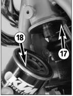
The screw @ must be removed to allow the motor oil to flow out of the frame breast pipe.
