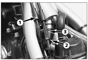
If a correction is necessary, start by removing the tank. Slide back the protection cover ①. To set the backlash, loosen the counter nut ② and turn the adjusting screw ③ accordingly. Then, fasten the counter nut and slide the protection cover back on.
