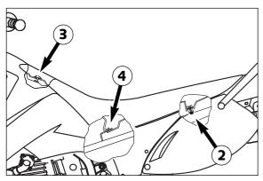
To mount the seat hook it into the oval head screw, lower the rear part of the seat and push the whole seat forwards. If necessary push the middle of the seat slightly down to let the retaining bracket ④ engage with the seat. Finally fasten the seat with the corresponding screw.
