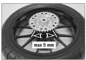
For this purpose, lie the rear wheel on a work bench with the rear sprocket upwards, and put the wheel spindle in the hub. Now hold the rear wheel firmly and try to turn the rear sprocket. The rear sprocket may not turn more than maximum 5 mm (0,2 in) measured on the outside. If the play in the chain wheel is larger, all 6 shock damping rubbers are to be replaced. Check the shock damping rubbers for signs of damage and dirt.
