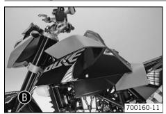
Remove the cloth **B** from between the compensating tank and the spoiler.
