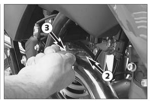
Loosen the allan head screw **1** at the adjustment ring **2**. Use the special wrench **3** from the tool set to turn the adjusting ring as required. Place the adjusting ring in a suitable position, and tighten the allan head screw with 8 Nm (6 ft.lb).
