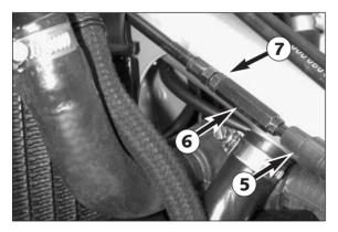
Push the choke lever all the way to the front and slide the protecting cap 6 from the adjusting part 6.
