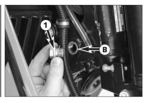
Fill 0.6 liters of engine oil into the can and remove the plug ① next to the steering head. Introduce the plastic hose into the vent hole ③, and fill 0.6 liters of engine oil into the frame's front tube. Remove plastic hose, start engine, and let it idle (approx. 20 seconds) until oil escapes at the hole ⑤. As soon as oil starts to escape, turn off the engine, and mount the plug together with the gasket.
