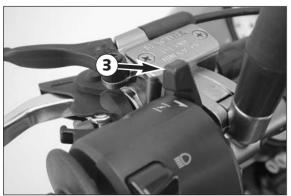
When the choke lever 3 is pulled backwards, a bore is opened in the carburetor which enables the engine to draw in additional fuel. This produces a "rich" fuel/air mixture necessary for cold start. When the choke lever is pushed forward as far as it will go, the bore will be closed again. In this position the choke cable must have a play of approx. 2 mm.
