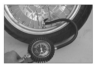
Tire pressure should be checked regularly on a "cold" tire. Proper pressure ensures optimum driving comfort and extends the life of your tires.
