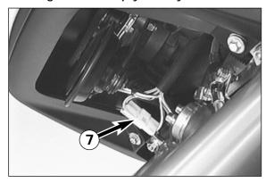
When the battery of the motorcycle is empty the engine can only startet by disconnecting the power supply of the head light. For this purpose a pin and socket connector • can be fund below the headlight mask. Disconnect the pin and socket connector and start the engine with the kickstarter.
