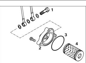
Check the O-ring § for damage. O-rings need not be replaced unless damaged. Press the O-ring into the groove of the filter cover. Fit new oil filter § with rubber gasket on the fitting in oil filter cover and mount cover with filter. Mount three screws and tighten with 5 Nm (4 ft.lb). Mount hollow screw with seal rings and tighten with 15 Nm (11 ft.lb). Start engine and check oil system for leakage.
