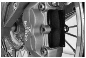
Insert new brake pads into the brake caliper, replace retainer spring (arrow pointing upward), and reinsert cotter bolt. Hammer the bolt into the caliper as far as it will go and replace cotter pin.
