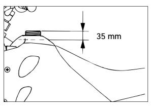
Fuel expands when its temperature rises. Therefore do not fill the tank to the top (see fig.).
