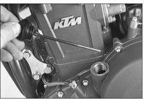
To allow the air to escape from the front pipe of the frame, remove plug next to the steering head. Start engine and let it run in idle (1-2 minutes) until oil escapes at the bore . As soon as oil starts to escape, turn off the engine, and mount plug together with the gasket.
