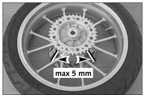
For this purpose, lie the rear wheel on a work bench with the rear sprocket upwards, and put the wheel spindle in the hub. Now hold the rear wheel firmly and try to turn the rear sprocket. The rear sprocket may not turn more than maximum 5 mm (0,2 in) measured on the outside. If the play in the chain wheel is larger, all 6 shock damping rubbers are to be replaced. Check the shock damping rubbers for signs of damage and dirt.
