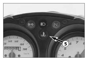
A mixture of 40% antifreezer and 60% water is used as cooling liquid. How-ever, the anti-freeze protection must be at least -25° C (-13° F). Aside from antifreezing protection, this mixture also provides great corrosion protection which is why it must not be replaced by pure water.
