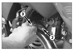
Loosen the allan head screw ① at the adjustment ring ②. Use the special wrench ③ from the tool set to turn the adjusting ring as required. Place the adjusting ring in a suitable position, and tighten the allan head screw with 8 Nm (6 ft.lb).
