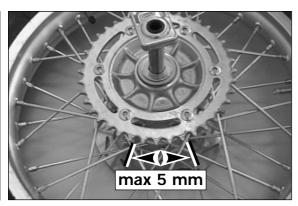
For this purpose, lie the rear wheel on a work bench with the rear sprocket upwards, and put the wheel spindle in the hub. Now hold the rear wheel firmly and try to turn the rear sprocket. The rear sprocket may not turn more than maximum 5 mm (0,2 in) measured on the outside. If the play in the chain wheel is larger, all 6 shock absorption rubbers are to be replaced. Check the shock absorption rubbers for signs of damage and dirt.
