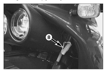
When the battery of the motorcycle is empty the engine can only be started by disconnecting the power supply of the head light. For this purpose a pin and socket connector ③ can be found below the headlight mask on the lefthand side. Disconnect the pin and socket connector and start the engine with the kickstarter
