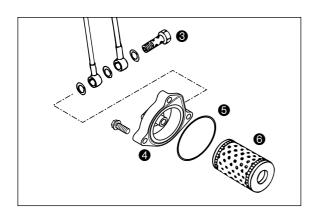
Check the O-ring for damage. O-rings need not be replaced unless damaged. Press the O-ring into the groove of the filter cover 4. Fit new oil filter with rubber gasket on the fitting in oil filter cover and mount cover with filter. Mount three screws and tighten with 5 Nm (4 ft.lb). Mount hollow screw with seal rings and tighten with 15 Nm (11 ft.lb). Start engine and check oil system for leakage.
