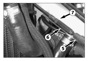
Push the choke lever all the way to the front and slide the protecting cap **6** from the adjusting part **6**.
