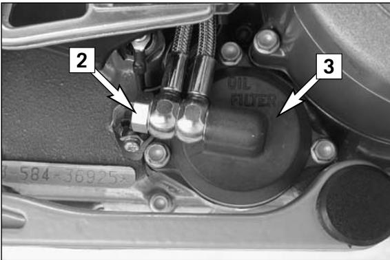
Place the new oil filter [4] on the connection in the oil filter cover and mount together with a new seal [5]. Tighten the 3 screws in the filter cover to 5 Nm. Tighten the hollow screw with seals and tighten to 15 Nm. Finally, start the engine and check the oil system for leakage.
