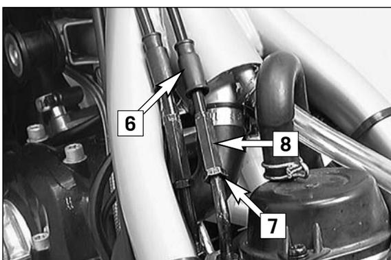
If a correction is necessary, start by removing the tank. Slide back the protection cover [6]. To set the backlash, loosen the counter nut [7] and turn the adjusting screw [8] accordingly. Then, fasten the counter nut and slide the protection cover back on.
