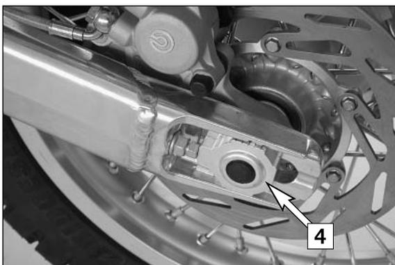
NOTE: The large adjusting range of the chain adjusters 32mm (1.28 in) allows you to use different secondary ratios in combination with the same chain length. The chain adjusters [4] can be rotated by 180°.
