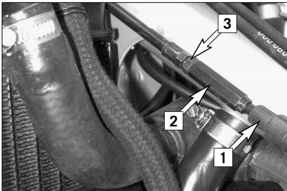
Push the choke lever all the way to the front and slide the protecting cap [1] from the adjusting part [2].
