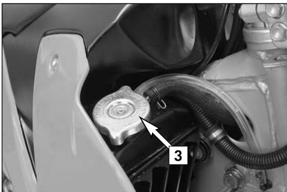
A mixture of 50% antifreeze and 50% water is used as cooling liquid. However, the anti-freeze protection must be at least -25°C (-13°F). Aside from antifreezing protection, this mixture also provides great corrosion protection which is why it must not be replaced by pure water.
