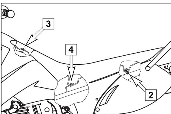
To mount the seat hook it into the oval head screw, lower the rear part of the seat and push the whole seat forwards. If necessary push the middle of the seat slightly down to let the retaining bracket [4] engage with the seat. Finally fasten the seat with the corresponding screw.
