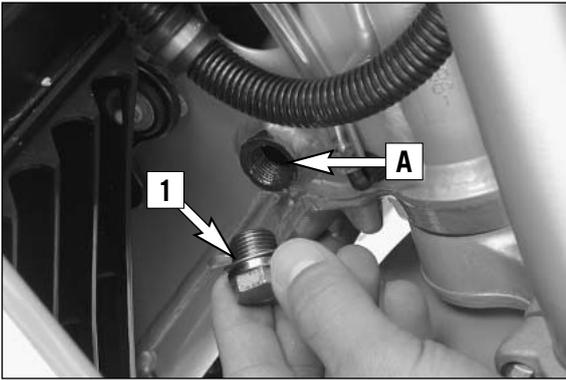
Fill 0.6 liters (0.16 US gallons) of engine oil into the can and remove the plug [1] next to the steering head. Introduce the plastic hose into the vent hole [A], (see page 30) and fill 0.6 liters (0.16 US gallons) of engine oil into the frame's front tube. Remove plastic hose, start engine, and let it idle (approx. 20 seconds) until oil escapes at the hole [A]. As soon as oil begins to leak out, switch off the engine, mount the plug and gasket and tighten to 25 Nm.
