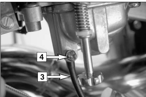
Open the drain plug [4] (turning it counterclockwise) by several turns, and drain the fuel from the float chamber.
