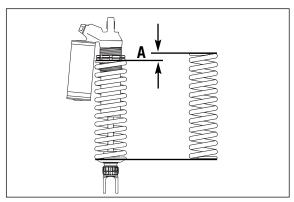
Loosen the locking ring [1] with the hook wrench from the tool set. Change the spring preload with the adjusting ring [2] and retighten the locking ring.
