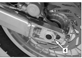
NOTE: The large adjusting range of the chain adjusters 32 mm (1.28 in) allows you to use different secondary ratios in combination with the same chain length. The chain adjusters [4] can be rotated by  $180^{\circ}$ .
