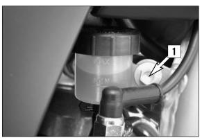
Refilling the rear brake fluid reservoir \*
