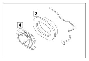
Mount the air filter on the filter holder, position in the filter box (make sure to center) and fix with the retaining clip. Check whether the air filter is positioned correctly and mount the filter box cover.
