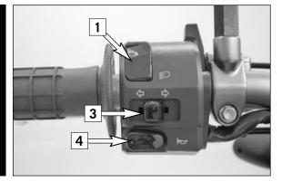
⇔ The indicator switch [3] returns to central position after actuation. Press flasher switch towards switch housing to switch off the flasher.
