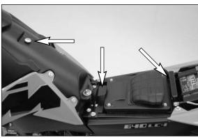
When you mount the seat, make sure the retaining brackets are fastened to the seat.
