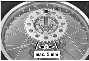
For this purpose, lie the rear wheel on a work bench with the rear sprocket upwards, and put the wheel spindle in the hub. Now hold the rear wheel firmly and try to turn the rear sprocket. The rear sprocket may not turn more than maximum 5 mm (0,2 in) measured on the outside. If the play in the chain wheel is larger, all 6 shock absorption rubbers are to be replaced. Check the shock absorption rubbers for signs of damage and dirt.
