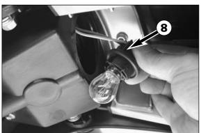
Turn the lamp socket 3 approximately 30° counterclockwise and pull it out of the tail light housing.
