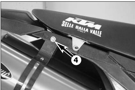
To remove the main silencer, remove screw ④ and pull the main silencer off towards the back.
