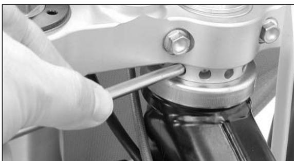
If the groove A is on the left, the offset is 12.5 mm and the caster 97.4 mm. This setting will give you better handling in curves.
