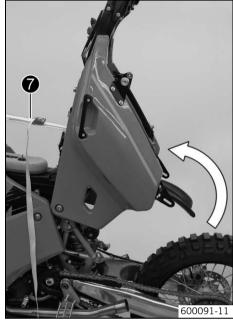
Fold the rear tank upward in the direction of the arrow and use a belt of to secure
