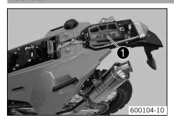
The tool set **1** is contained in the accessories box and can be stored in the compartment beneath the additional lamps.
