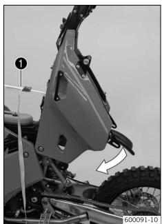
Detach the belt 1 and carefully position the rear tank.
