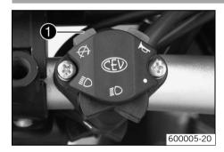
The short circuit button • is fitted on the left side of the handlebar and has no function upon delivery.
