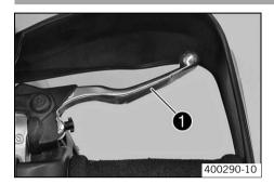
The hand brake lever **1** is located on the right side of the handlebar and operates the front wheel brake.
