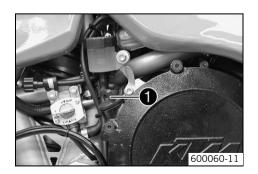
Remove the screw cap • on the clutch cover and fill up with engine oil.
