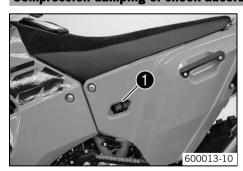
The compression damping can be adjusted via an opening **1** on the left side of the rear tank.
