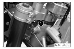
The steering lock • is fitted on the left of the steering head.
