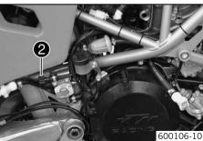
The idle speed is adjusted with the adjustment screw 2.
