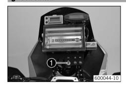
The ignition switch **1** is located to the left of the indicator lamp on the instrument support.
