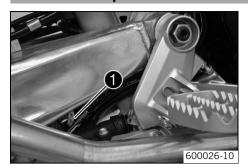
Shock absorber part number lacktriangle is attached at the shock absorber unit, to the rear of the direction of travel.
