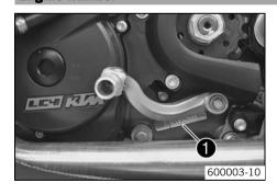
The engine number  $oldsymbol{0}$  is stamped on the left side of the engine under the engine sprocket.
