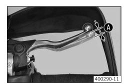
Pull the hand brake lever and check the free travel .
