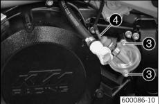
Mount and tighten screws 3.
