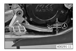
Move the foot brake lever backwards and forwards between the end stop and the foot brake cylinder piston bracket and check free play .
