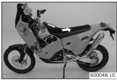
Carefully push the seat to the rear and remove it.
