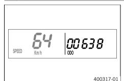
Press the button D briefly and repeatedly until ODO appears at the bottom right of the display.
