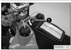
Lift the quick-locking clip ● and rotate in the direction of the arrow.
