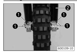
Position the front fender ②. Mount and tighten screws ①.
