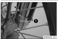
The fork part number lacktriangle is stamped on the inner side of the fork stub.
