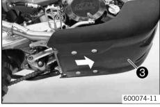
Pull the motor guard 3 forward out of the frame.
