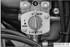
• **R REAR** – If tap handle **4** of the fuel tap points up, fuel is taken from the rear fuel tank. Only the rear fuel tank empties out completely.
