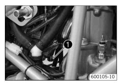
The idle mixture is adjusted with the idle mixture adjustment screw **①**.
