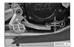
Move the foot brake lever backwards and forwards between the end stop and the foot brake cylinder piston bracket and check free play .
