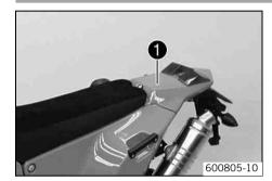
The tool set is contained in the accessories box and can be stored in compartment **1** beneath the additional lamps.
