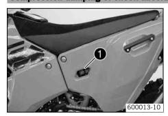
The compression damping can be adjusted via opening **1** on the left side of the rear tank.
