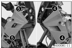
Align the trim and attach it with the quick releases 4 and 5.
