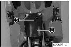
Position the splash protector **6**. Mount and tighten screws **6**.
