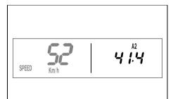
**A2** (average speed 2) shows the average speed on the basis of the current speed if the stop watch **S2** (stop watch 2) is running.
