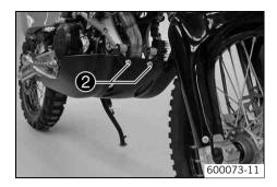
Mount and tighten screws ②.
