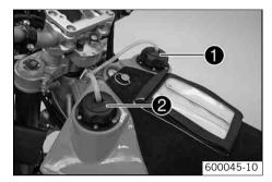
This model has three separate fuel tanks controlled by a fuel tap. Two fuel tanks are located in front of the seat and one fuel tank is located beneath the seat.
