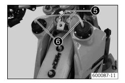
Mount and tighten screws 6.
