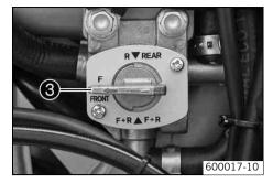
• **F FRONT** – If tap handle **③** of the fuel tap points toward the rear, fuel is taken from the two front fuel tanks. Only the front fuel tanks empty out completely.
