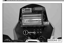
The ignition switch lacktriangle is located to the left of the indicator lamp on the instrument support.
