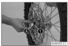
Clean and grease shaft seal ring • and bearing surface • of the distance bushing. Clean and grease the shaft seal ring on the right and the running surface of the wheel spindle.
