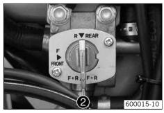
• **F+R** – If tap handle ② of the fuel tap points down, fuel is taken from all three fuel tanks. All fuel tanks empty out completely.
