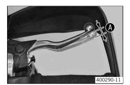
Pull the hand brake lever and check the free travel .
