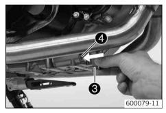
Fit and tighten plug 3 with oil screen 4 and O-ring.
