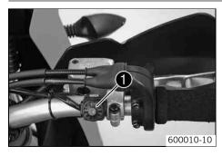
The electric starter button **①** is fitted on the right side of the handlebar.
