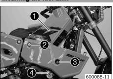
Position the fuel tank ● on the left and right. Mount and tighten screws ② and ⑤ on the left and right.
