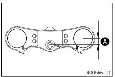
The fork offset **4** has an impact on the handling of the vehicle. It is calculated from the center of the fork leg to the center of the steering head bearing. The fork offset can optionally be adjusted.
