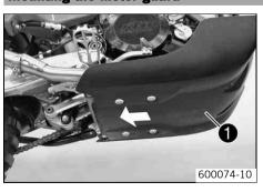
Insert the motor guard 1 into the frame.
