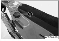
The rear fuel tank is filled via filler cap 3.
