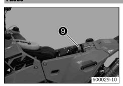
The fuse box  $\ensuremath{\mathbf{9}}$  is located under the seat.
