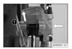
Press the brake caliper by hand on to the brake disc in order to press back the brake piston.
