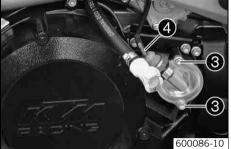
Mount and tighten screws 3.
