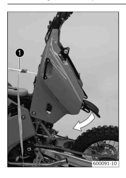
Detach the belt • and carefully position the rear tank.
