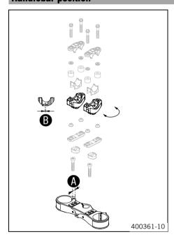
On the upper triple clamp, there are 2 holes at a distance of **3** to each other.
