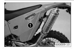
There is one handrail • attached at the left and one at the right (at the rear tank). The handrail is used for shunting the motorcycle.
