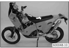
Carefully push the seat to the rear and remove it.
