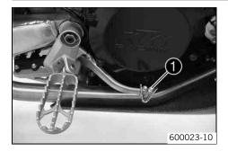
Foot brake pedal **1** is located in front of the right footrest. The rear brake is engaged with the foot brake pedal.
