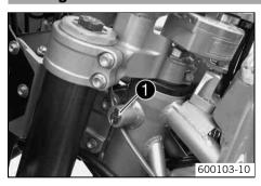
The steering lock • is fitted on the left of the steering head.
