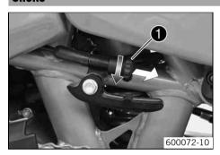
The choke knob • is fitted on the left side of the frame.
