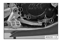
Loosen the nut • and use the screw • to adjust the free travel •.
