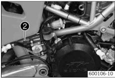
The idle speed is adjusted with the adjustment screw 2.
