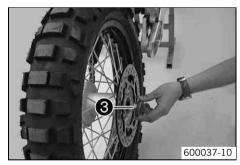
Remove the rear sprocket carrier 4.
