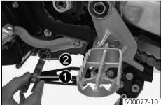
Fit and tighten plug • with oil screen • and O-ring.
