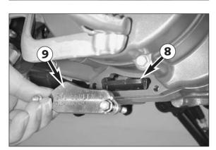
Mount the oil drain plug on the engine with a new seal ring and tighten to 20  $\mbox{Nm}.$
