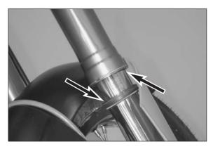
Clean dust-protection bellows, outer tubes, and fork tubes thoroughly, and oil them thoroughly with silicone spray. Then, push dust-protection bellows into the outer tubes by hand.
