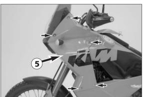
Remove the **5** screws, take off the left panel 5 and disconnect the turn signal cable.
