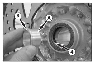
Before remounting the front wheel, clean and grease the shaft seal rings **4** and the bearing surface **4** of the distance bushings and mount the distance bushings (wide distance bushing in the left shaft seal ring). Slightly push back the brake pads with a screwdriver. Position the front wheel against the brake disks according to the direction of travel (see arrow **6**).
