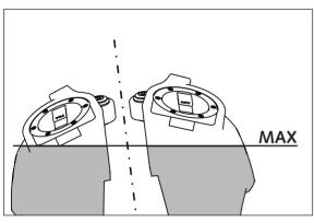
The 950 Adventure has 2 tanks with 1 filler neck each. Fill the right tank first, then the left tank (see drawing for the maximum filling level). If the right tank is filled up to the filler neck, fuel may overflow when the motorcycle is parked on the side stand after refueling when the fuel becomes warm.
