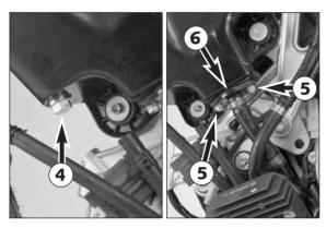
Remove the drain plug **4** on the oil tank and allow the oil to drain into a receptacle. Remove the screws **6** and tilt the oil return valve **6** to the side.
