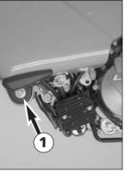
Remove the 3 screws ①, lift the tank approx. 15 mm and carefully tilt to the side. Disconnect the connector from the pickup cable (fuel level) and set the tank down.
