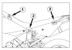
To remount, fit the nose **①** of the seat in the front, lower the back while pushing towards the front. Both noses **②** should fit into the frame. Insert the catch bolts **③** in the lock housing and push the seat down in the back until you hear the catch bolts snap into place. Check whether the seat is correctly mounted.
