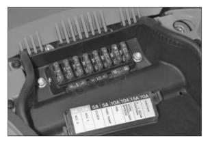
Replace a blown fuse only with an equivalent one. If a new fuse that has just been set in gets blown again, you are strongly advised to have it inspected by a KTM dealer.
