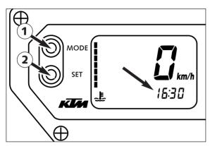
Switch on the ignition and change to the CLOCK mode.
