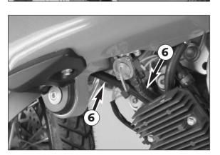
Close all 3 fuel taps and the disconnect the fuel lines **6** from the left tank.
