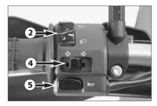
The indicator switch 4 returns to central position after actuation. Press flasher switch towards switch housing to switch off the flasher.
