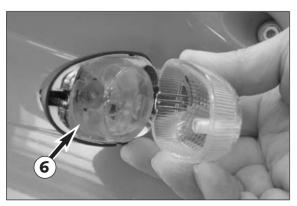
Slightly depress the bulb, turn it approx.  $30^{\circ}$  counterclockwise and pull it out of the socket.
