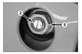
The adjusting screw 2 for the low-speed range can be adjusted with a screwdriver.
