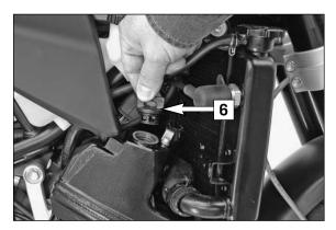
Add 2.5 liters (0.7 USgal) of fully synthetic engine oil meeting the JASO MA standard (e.g. Motorex Power Synt 4T) and mount the oil dipstick [6]. Start the engine, allow to run warm for 4 minutes and switch off the engine. Remove the oil dipstick and add engine oil up to the MAX mark (approx. 0.5 liters, 0.13 USgal).
