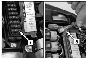
The ACC fuse [7] is designed for accessories with a maximum power consumption of 10 amperes. A connector [8] to connect the equipment is provided under the seat. Ask your authorized KTM workshop for details.
