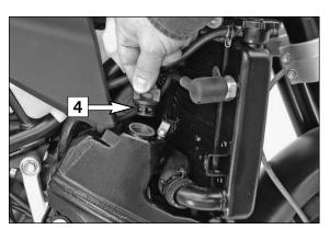
Unscrew the plug [4] and refill engine oil. Wait 20 seconds and check the oil level again. The quantity of oil between the MIN and MAX marks is 0.3 liter. Mount the plug and check the engine for leaks. Finally, mount the spoilers.
