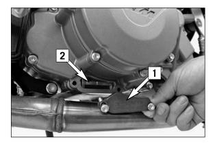
Mount the oil drain plug on the engine with a new seal ring and tighten to  $20\ \text{Nm}.$
