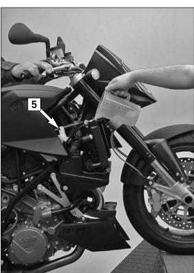
To completely bleed the cooling system, the motorcycle must be raised approx. 50 cm in the front.
