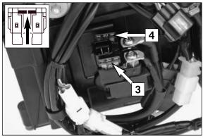
Pull the connector [1] out of the bracket, remove the cap [2] and check the main fuse [3]. A spare fuse [4](30 amperes) is also plugged into the bracket. Always replace blown fuses with an equivalent fuse. Visit an authorized KTM workshop if a new fuse blows again after it is inserted.
