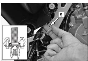
Carefully pull the oil screen [9] out of the oil tank.
