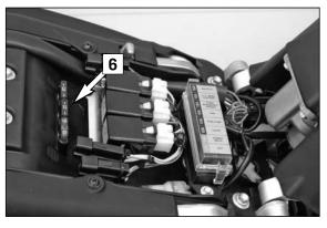
Replace a blown fuse only with an equivalent one. If a new fuse that has just been set in gets blown again, you are strongly advised to have it inspected by a KTM dealer.
