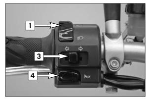
中中 The indicator switch [3] returns to central position after actuation. Press flasher switch towards switch housing to switch off the flasher.
