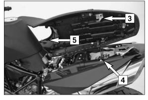
To mount the seat, place it on the motorcycle and position the hooks [3] on the bottom of the seat behind the dollies [4] on the subframe. Press down on the seat near the holding strap while sliding it forwards. The two tabs [5] must hook onto the tank. Turn the ignition key in the seat lock 90° in a counterclockwise direction and pull off. Check whether the seat is mounted correctly.
