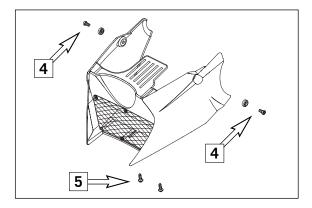
Remove the screws [4], loosen the screws [5] by 2 turns and remove the front spoiler towards the front.
