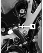
Mount the oil drain plug on the oil tank with a new seal ring and tighten to 20 Nm.
