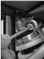
The adjusting screw [1] for the low-speed range can be adjusted with a screwdriver.
