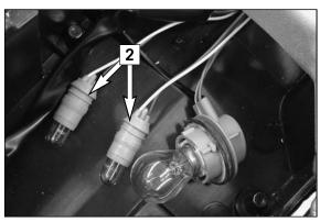
BULBS FOR THE TAILLIGHT: Remove the bulb socket [2] from the housing and pull the bulb out of the socket. Insert a new bulb and press the bulb socket all the way into the taillight housing.
