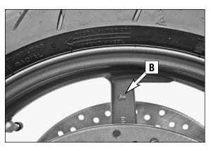
Before you remount the front wheel, clean and grease the shaft seal rings [5] and the bearing surface [A] of the distance bushings and mount the distance bushings (wide distance bushing in the left shaft seal ring). When mounting the distance bushing, be careful not to press the sealing lips towards the inside. position the front wheel according to the running direction shown by the arrows [B] on the rim.
