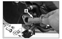
Carefully pull the oil screen [8] out of the oil tank.
