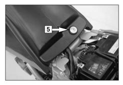
Remove the seat and screw [5]. Close the fuel taps and fuel line. Slightly pull the tank towards the back, lift about 10 cm (4 in) in the front and slide it under the tank a little bit to hold it in this position.
