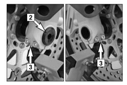
Loosen the collar screw [2] and the clamping screws [3] on both fork leg axle passages. Unscrew the collar screw approx 8 turns, press on the collar screw with your hand to push the wheel spindle out of the fork leg axle passage and remove the collar screw. Hold the front wheel while you pull out the wheel spindle. Lift the front wheel off the fork.
