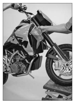
Add cooling liquid until it runs out of the vent holes without bubbles and immediately mount the screw to prevent air from entering the radiator.
