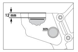
Fill DOT 5.1 brake fluid (Motorex Brake Fluid DOT 5.1) up to 12 mm (0.5 in) under the top edge of the reservoir. Remount the rubber boot, cover and screws. Wash off any overflowing or spilled brake fluid with water. Actuate the rear brake until you feel the point of pressure.
