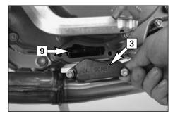
Mount the oil drain plug on the engine with a new seal ring and tighten to 20 Nm.
