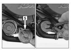
Changing the engine oil and the oil filter, cleaning the oil screen
