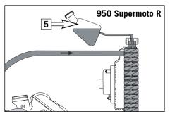
A mixture of 50% antifreeze and 50% distilled water is used as the cooling liquid. However, the anti-freeze protection must be at least  $-25^{\circ}$  C ( $-13^{\circ}$  F). Aside from antifreezing protection, this mixture also provides great corrosion protection which is why it must not be replaced by pure water.
