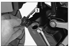
Unscrew the plug [3]. Add 2.5 liters (0.7 USgal) of fully synthetic engine oil according to the JASO MA Norm (e.g. Motorex Power Synt 4T) and remount the plug. Start the engine and allow to run warm in neutral until 4 bars on the temperature indicator light up. Switch off the engine and check the engine oil level (see Checking the engine oil level).
