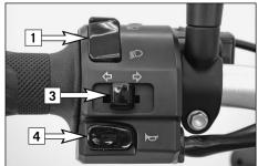
The indicator switch [3] returns to central position after actuation. Press flasher switch  $\Diamond \Diamond$ towards switch housing to switch off the flasher.
