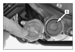
Insert a new oil filter [1] in the engine case, grease the O-ring and mount the oil filter cover together with the O-ring. Tighten the screws to 6 Nm.
