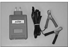
To charge the battery while mounted, always use the KTM battery charger (Item no. 58429074000) to ensure that the electric system is not damaged by excess voltage. **Always remove the battery if using other battery chargers!** You can also use this charging device to test the off-load voltage and startability of the battery and generator. It is impossible to overcharge the battery with this device.
