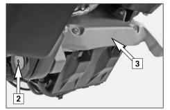
Remove the lower screw [2] on the right tank. Remove the HH screws and take off the battery cover [3].
