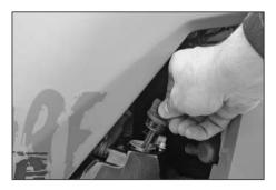
Add 2.5 liters (0.7 USgal) of fully synthetic engine oil meeting the JASO MA standard (e.g. Motorex Power Synt 4T) and mount the oil dipstick. Start the engine, allow to run warm for 4 minutes and switch off the engine. Remove the oil dipstick and add engine oil up to the MAX mark (approx. 0.5 liters, 0.13 USgal).
