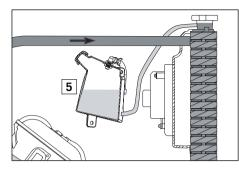
A mixture of 50% antifreeze and 50% distilled water is used as the cooling liquid. How ever, the anti-freeze protection must be at least  $-25^{\circ}$  C ( $-13^{\circ}$  F). Aside from antifreezing protection, this mixture also provides great corrosion protection which is why it must not be replaced by pure water.
