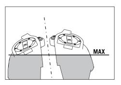
The 990 Adventure has 2 tanks with 1 filler cap each. Both filler caps can be locked and are equipped with a tank vent system. To open, insert the ignition key, turn  $45^{\circ}$  in a clockwise direction and fold up the filler cap. The ignition key can be pulled out to open the other filler cap. Simply press on the filler cap to close.
