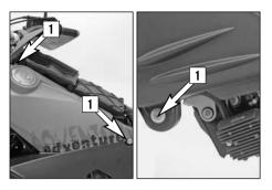
Remove the 3 screws [1], lift the tank approx. 15 mm and carefully tilt to the side. Disconnect the fuel lines, disconnect the connector for the fuel pump and the pickup cable (fuel level) and set down the tank.
