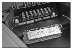
Replace a blown fuse only with an equivalent one. Visit an authorized KTM workshop if the new fuse blows again.
