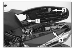
To mount the seat, place it on the motorcycle and position the hooks **[2]** on the bottom of the seat behind the dollies **[3]** on the subframe. Press down on the seat near the holding strap while sliding it forwards. The two tabs **[4]** must hook onto the tank. Turn the ignition key in the seat lock 90° in a counterclockwise direction and pull off. Check whether the seat is mounted correctly.
