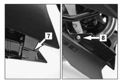
Fit the slots in the front spoiler on the lower screws **[7]** and tighten. Apply Loctite 243 to the side screws **[8]** and tighten to 10 Nm.
