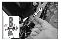
Carefully pull the oil screen [9] out of the oil tank.
