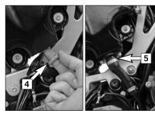
Mount the oil drain plug on the oil tank with a new seal ring and tighten to 20 Nm.
