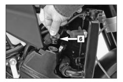
Remove the right spoiler (see Refilling the engine oil) and unscrew the plug **[6]**. Add 2.5 liters (0.7 USgal) of fully synthetic engine oil meeting the JASO MA standard (e.g. Motorex Power Synt 4T) and remount the plug. Start the engine and allow to run warm in neutral until 4 bars on the temperature indicator light up. Switch off the engine and check the oil level (see Checking the engine oil level).
