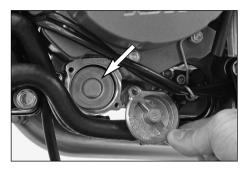
Insert a new oil filter in the engine case, grease the O-ring and mount the oil filter cover together with the O-ring. Tighten the screws to 6 Nm.
