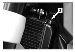
Add cooling liquid until it runs out of the vent holes without bubbles and immediately mount the screw to prevent air from entering the radiator.
