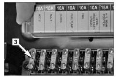
Fuses ACC 1 and ACC 2 [3] are designed for accessories with a maximum power consumption of 10 amperes each. Fuse ACC 2 also protects the carburetor heaters from short circuits.
