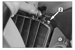
Add cooling liquid until it runs out of the vent holes without bubbles and immediately mount the screw to prevent air from entering the radiator.
