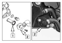
Mount the oil drain plug on the oil tank with a new seal ring and tighten to 20 Nm.
