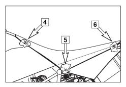
To mount the seat, attach the seat to the oval head screw [4], lower the seat in the back while sliding it towards the front. Both noses [5] should fit into the frame. Insert the catch bolts [6] in the lock housing and push the seat down in the back until you hear the catch bolts snap into place.
