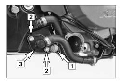
Remove the drain plug [1] from the oil tank and allow the oil to drain into a vessel. Remove the screws [2] and tilt the connector [3] to the side.
