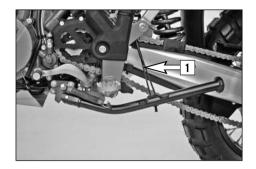
For off-road riding, you can use the rubber band [1] to additionally secure the center stand in its folded-up position
