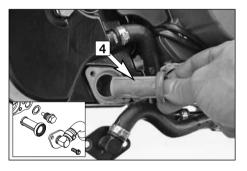
Carefully pull the oil screen [4] out of the oil tank.
