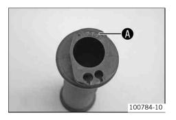
The throttle grips can be distinguished by the markings stamped  $\bullet$  into the inner face. The installed throttle grip has the marking **3081**.
