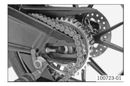
Push the rear wheel as far forward as possible and then remove the chain from the rear sprocket.
