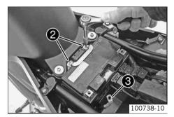
Mount and tighten screws ②.
