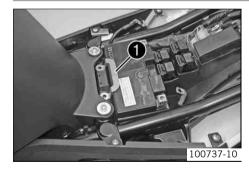
Position the battery in the battery rack.
