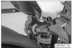
When you screw in the rear left fixing screw, the plug-in cable binder • is pushed out of the thread. To reposition the cable of the lambda probe, fix the plug-in cable binder in the remaining free drill hole.
