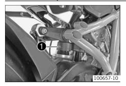
The shock absorber part number lacktriangle is stamped on the upper part of the shock absorber above the adjusting ring towards the rear.
