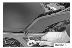
Mount the screw and washer on the left and right sides of the vehicle, but do not tighten.
