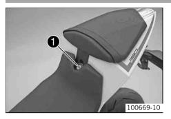
The seat lock **①** is behind the seat. It can be locked with the ignition key.
