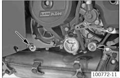
Mount and tighten the oil drain plugs with the magnet, O-rings and oil screen.
