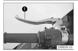
The clutch lever **1** is fitted on the left side of the handlebar. The clutch is hydraulic and self-adjusting.
