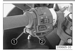
The **MODE** button **1** is fitted on the handlebar, front left.
