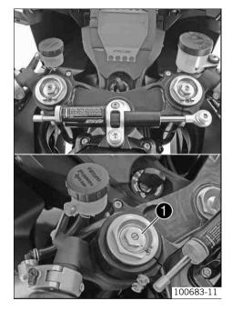
Turn adjusting screws 1 clockwise to the stop.
