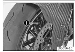
The fork part number • is stamped on the inner side of the fork stub.
