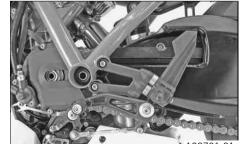
Mount and tighten screws.
