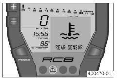
**REAR SENSOR** appears on the info display if the rear cylinder coolant temperature sensor is faulty.
