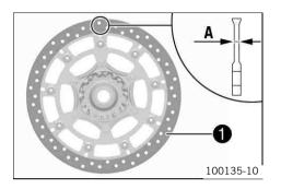
Check the thickness of the brake disc in several places to see if it is within the specified wear tolerance .
