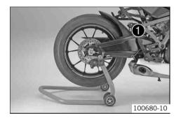
Insert the work stand adapter in the rear of the work stand.
