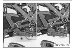
The adjustable footrest system enables an individual setting of the footrest height and an individual adjustment of the operating elements.
