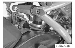
Turn the adjusting ring counterclockwise with the wrench from the tool kit until the spring is no longer under tension.
