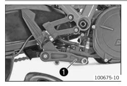
The foot brake pedal **1** is in front of the right footrest. The foot brake pedal operates the rear brake.
