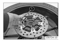
Remove spacer ①. Clean and grease the mating surfaces of the spacers and the shaft seal rings.
