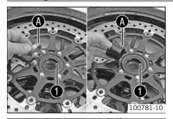
Clean and grease the shaft seal rings ● and mating surfaces ● of the spacers.
