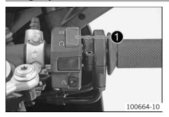
The emergency OFF switch • is installed on the right side of the handlebar.
