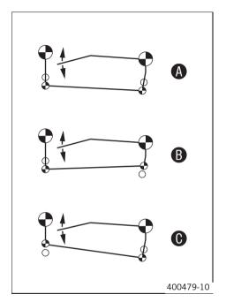
The shift rod can be mounted both on the shift lever variably at an upper or lower position, and on the reverse gear change of the shift shaft in two different positions.
