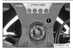
The ignition/steering lock **1** is located in front of the upper triple clamp.
