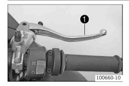
The hand brake lever **①** is fitted on the right side of the handlebar. The hand brake lever operates the front brake.
