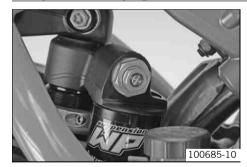
The shock absorber can regulate compression damping separately in the low and high speed ranges (Dual Compression Control).
