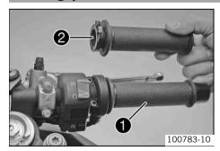
The installed throttle grip • twists opens uniformly (linear) over the entire range of the throttle valve.
