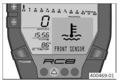
**FRONT SENSOR** appears on the info display if the front cylinder coolant temperature sensor is faulty.
