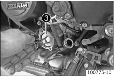
Pull oil filter 3 out of the oil filter housing.
