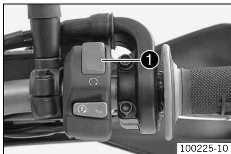
The emergency OFF switch ❶ is fitted on the right side of the handlebar.
