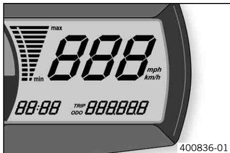
When you switch on the ignition, all display segments light up for one second as a function test.
