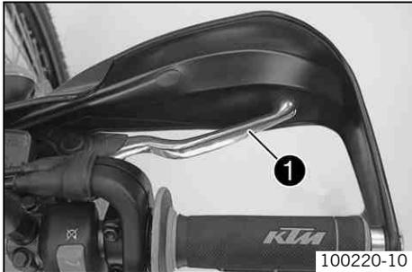
The hand brake lever ❶ is fitted on the right side of the handlebar.
