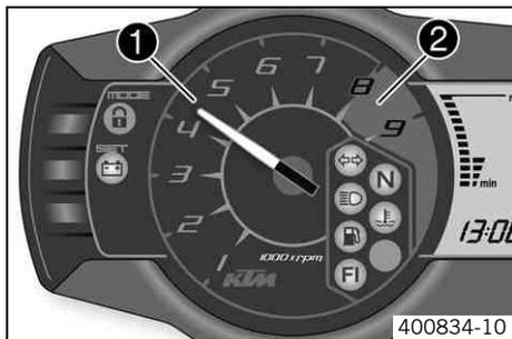
The tachometer ❶ shows the engine speed in revolutions per minute. The red marking ❷ shows the excess speed range of the engine.
