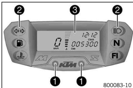
The combination instrument is installed in front of the handlebar. The combination instrument is divided into 3 function areas.
