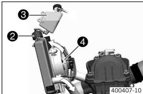
Cooling takes place by means of the air stream and a radiator fan ④, which is controlled by a thermostat.
