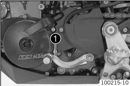
The shift lever ❶ is mounted on the left side of the engine.
