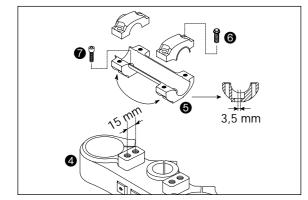
For this purpose, remove screws ③ of the handlebar clamps and screws ④ of the handlebar support. Position handlebar support, and tighten screws ④ to 40 Nm (30 ft.lbs). Mount handlebar and handlebar clamps, and tighten screws ⑤ to 20 Nm (15 ft.lbs). The gap between handlebar support and handlebar clamps is to be of equal size in the front and in the rear.
