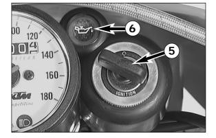
The red oil level warning lamp 6 lights up when the ignition is swit-<del>متہ</del> ched on, indicating that the oil level warning system works properly.
