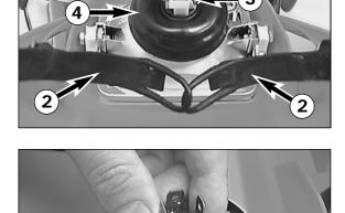
Insert a new bulb such that the noses 3 fit into the recess 3. Do not touch the glass body of the bulb, to keep if free from grease. Mount supporting ring, rubber cap and plug. Position headlight mask with the bottom holders, and fasten it with the rubber bands 3.
