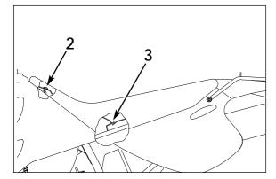
Mounting the seat: Hook the seat onto the oval head screw 2. Slide it forward to let the retaining plate 3 engage in the seat. Slide retaining shackles of seat under the side covers and mount screws 1
