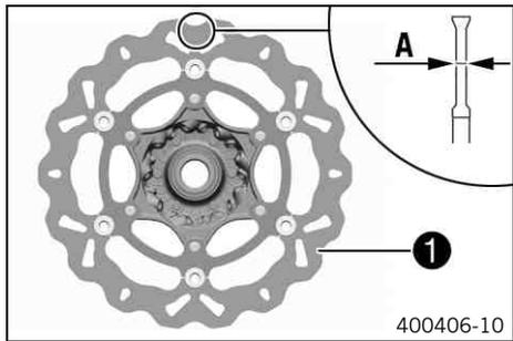
– Check the thickness of the front and rear brake discs in several places to ensure that it conforms to measurement **A**.
