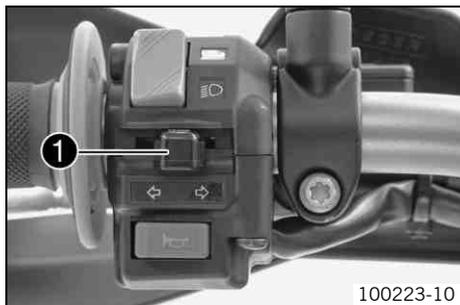
The turn signal switch ❶ is fitted on the left side of the handlebar.
