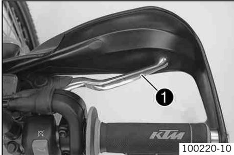
The hand break lever ❶ is fitted on the right side of the handlebar.
