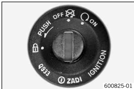
The ignition/steering lock ❶ is located in front of the seat.
