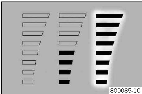
The temperature display consists of 8 bars. The more bars that light up, the hotter the coolant. When the upper bar lights up, all bars in the display begin to flash and the temperature warning lamp lights up.
