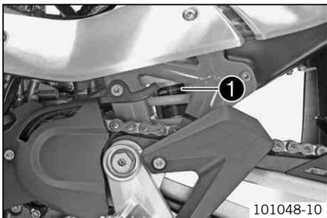
The shock absorber part number ❶ is on the left of the shock absorber.
