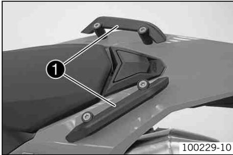
The handrails ❶ are used for moving the motorcycle around.
