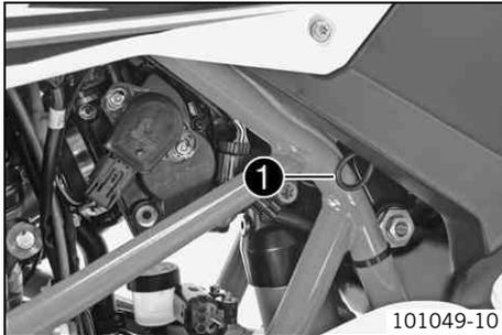
The seat can be released using strap ❶.
