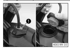
Press release button 1, turn filler cap counterclockwise and lift it upwards and remove.
