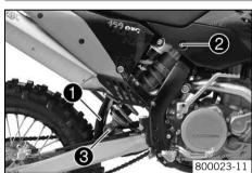
Push splash protector • to the side and position the shock absorber. Mount and tighten screw •.
