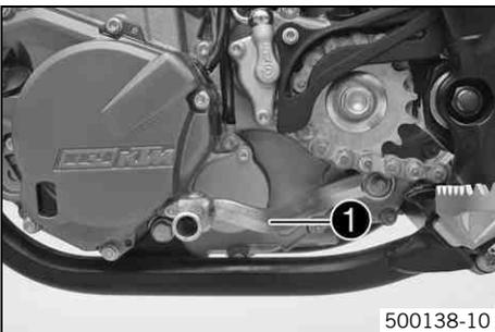
Shift lever ❶ is mounted on the left side of the engine.
