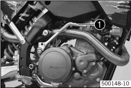
The kick starter ❶ is fitted on the right of the engine. The engine can be started with either the kick starter or the electric starter. The upper part of the kick starter can be swung out.
