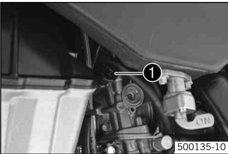
Choke ❶ is fitted on the left side of the carburetor.
