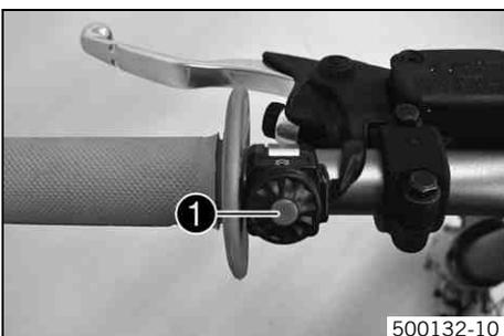
The short circuit button ❶ is fitted on the left side of the handlebar.
