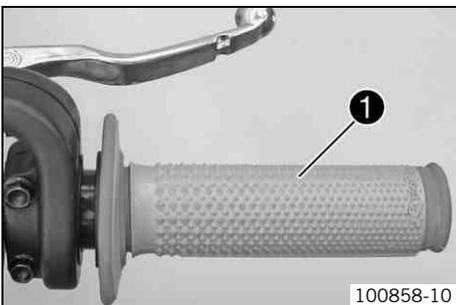
The throttle grip ❶ is fitted on the right side of the handlebar.
