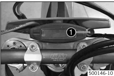
The light switch ❶ is on the right of the speedometer.
