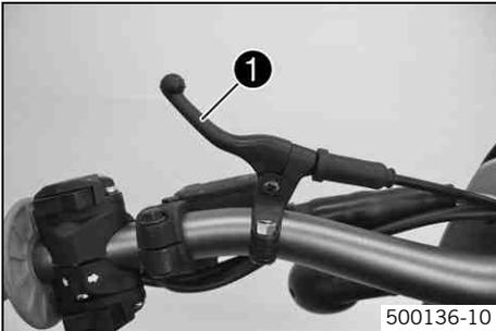
The choke lever ❶ is fitted on the left side of the handlebar. Activating the choke function frees an opening through which the engine can draw extra fuel. This gives a richer fuel-air mixture, which is needed for a cold start.
