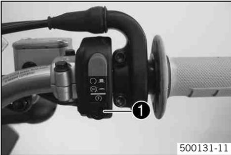
The electric starter button ❶ is fitted on the right side of the handlebar.
