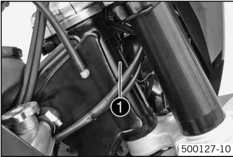
The chassis number ❶ is stamped on the steering head on the right.
