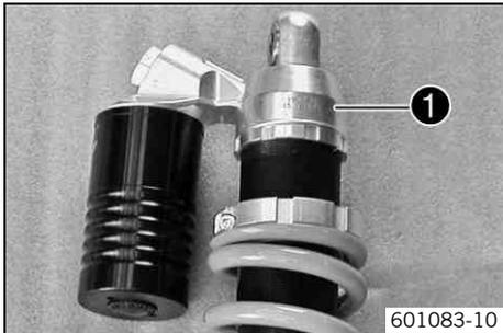
The setting number ❶ is stamped into the top of the shock absorber.
