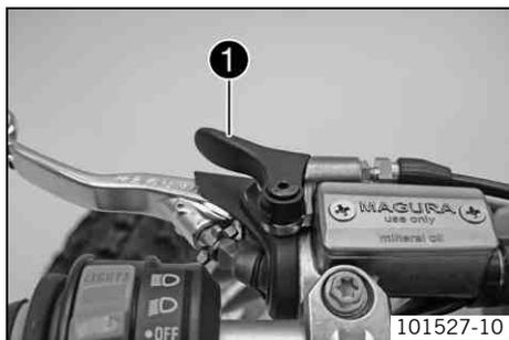
The reverse gear release lever ❶ is fitted on the left side of the handlebar. Reverse gear can only be engaged when the reverse gear release lever is activated while the vehicle is at a standstill.
