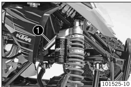
The type label ❶ is located on the frame tube on the right in front of the radiator.
