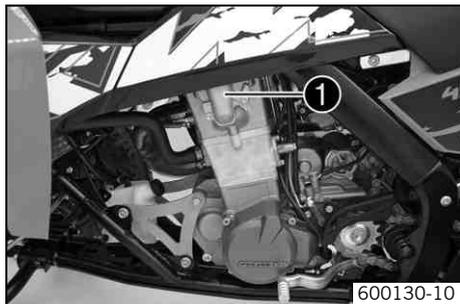
The water pump ❶ in the engine forces the coolant to flow. The pressure resulting from the warming of the cooling system is regulated by a valve in the radiator cap . This ensures that operating the vehicle at the specified coolant temperature will not result in a risk of malfunctions.
