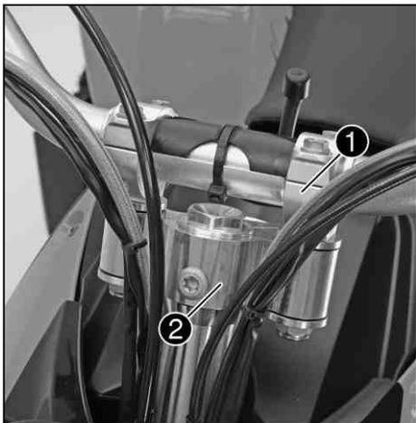
The handlebar position can be adjusted 4-fold by turning the handlebar support **1** and the handlebar support **2**.
