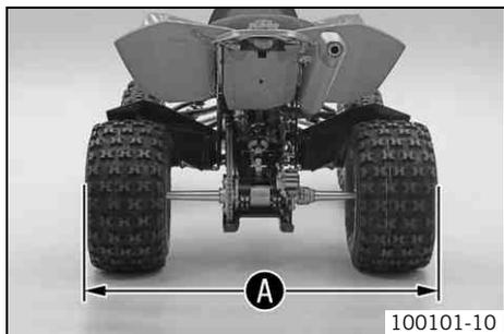
The toe width **A** can be adjusted by installing the spacer in various ways.
