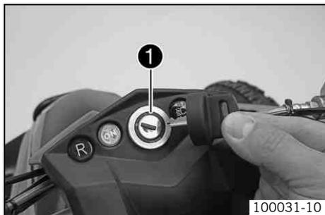
The ignition lock ❶ is located on the instrument support.
