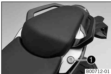
The seat lock ❶ is located to the left of the seat. It can be locked with the ignition key.
