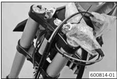
Route the clutch line with the clutch master cylinder toward the front between the upper and lower triple clamps.
