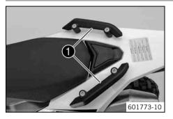
The handrails  $\bullet$  are used for moving the motorcycle around. When you have a passenger, the passenger can hold on the handrails during the journey.
