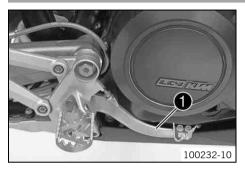
Foot brake lever  $\bullet$  is located in front of the right footrest. The rear brake is engaged with the foot brake lever.
