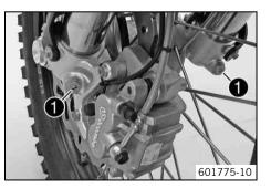
– Turn adjusting screws **1** clockwise all the way.
