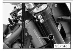
The chassis number  $\bullet$  is stamped on the steering head on the right.
