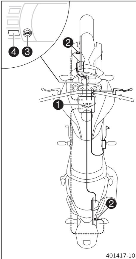
The ABS unit ❶, which consists of a hydraulic unit, ABS control unit, and return pump, is installed under the seat. A wheel speed sensor ❷ is located at the front and rear wheels.
