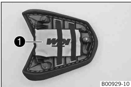
The tool set ❶ is located under the passenger seat.
