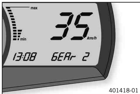
In display mode **GEAR**, the gear currently engaged is displayed.
