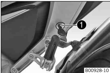
The seat lock ❶ is located on the left side of the vehicle. It can be locked with the ignition key.
