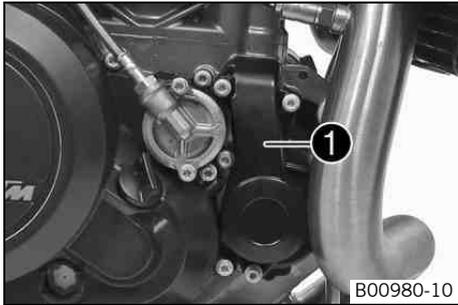
The water pump ❶ in the engine forces the coolant to flow.
