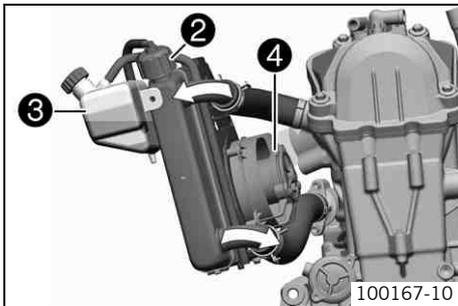
Cooling takes place by means of the air stream and a radiator fan ❹, which is controlled by a thermostwitch.
