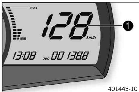
The speed ❶ is shown in kilometers per hour **km/h** or in miles per hour **mph**.
