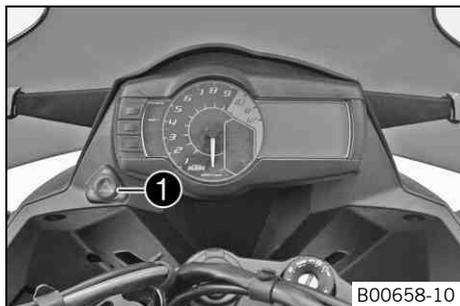
The hazard warning flasher switch ❶ is fitted next to the combination instrument on the left.
