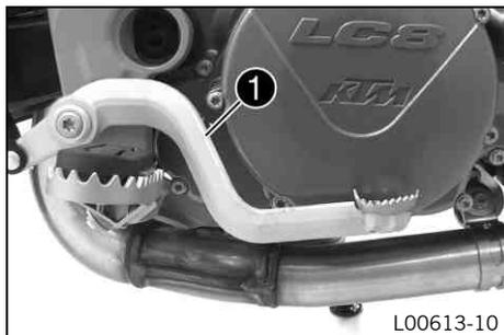
Foot brake lever ❶ is located in front of the right footrest. The rear brake is activated using the foot brake lever.
