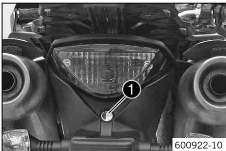
Seat lock ❶ is located at the rear under the tail light. It can be locked with the ignition key.
