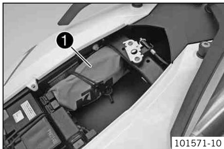
The tool set ❶ is located in the storage compartment under the seat.
