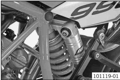
The compression damping of the shock absorber is divided into two ranges: high-speed and low-speed.
