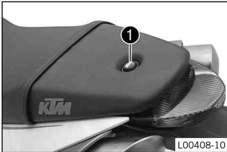
Seat lock ❶ is located at the rear of the seat. It can be locked with the ignition key.
