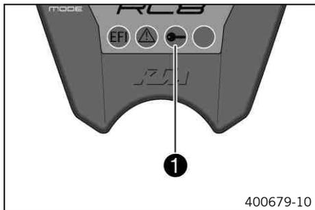
The electronic immobilizer secures the vehicle against unauthorized use. The immobilizer is activated automatically and the engine electronics are locked when the ignition key is withdrawn.
