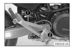
Position the footrest bracket ①. Mount and tighten screws ②.
