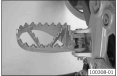
Mount the footrests with the springs and bolts. Secure the bolts using the washers and pins.
